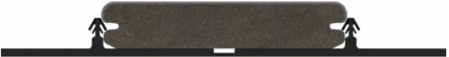
Snap-loc clip profile for Trex™ decking
