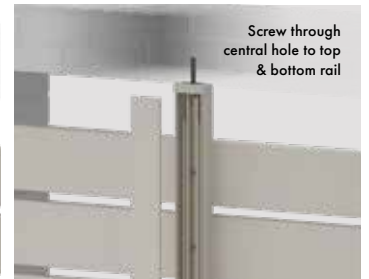
Screw top/bottom plate to centre support rail
