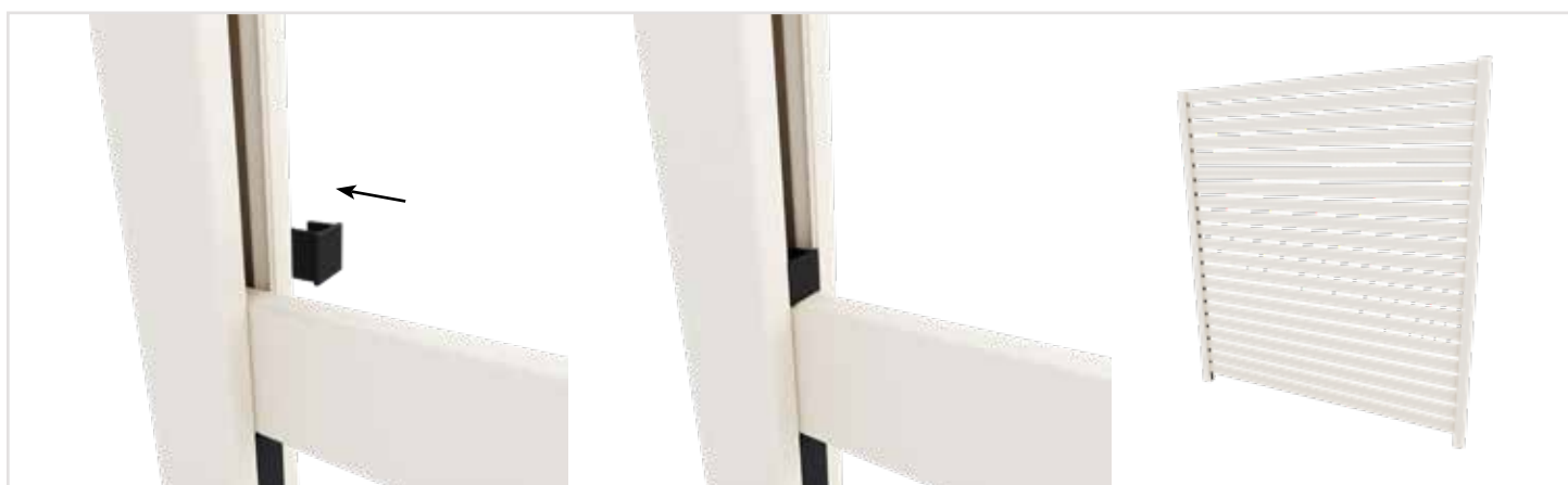
8 Snap in spacer block above first slat into either side of pocket of post. Repeat for all slats.
