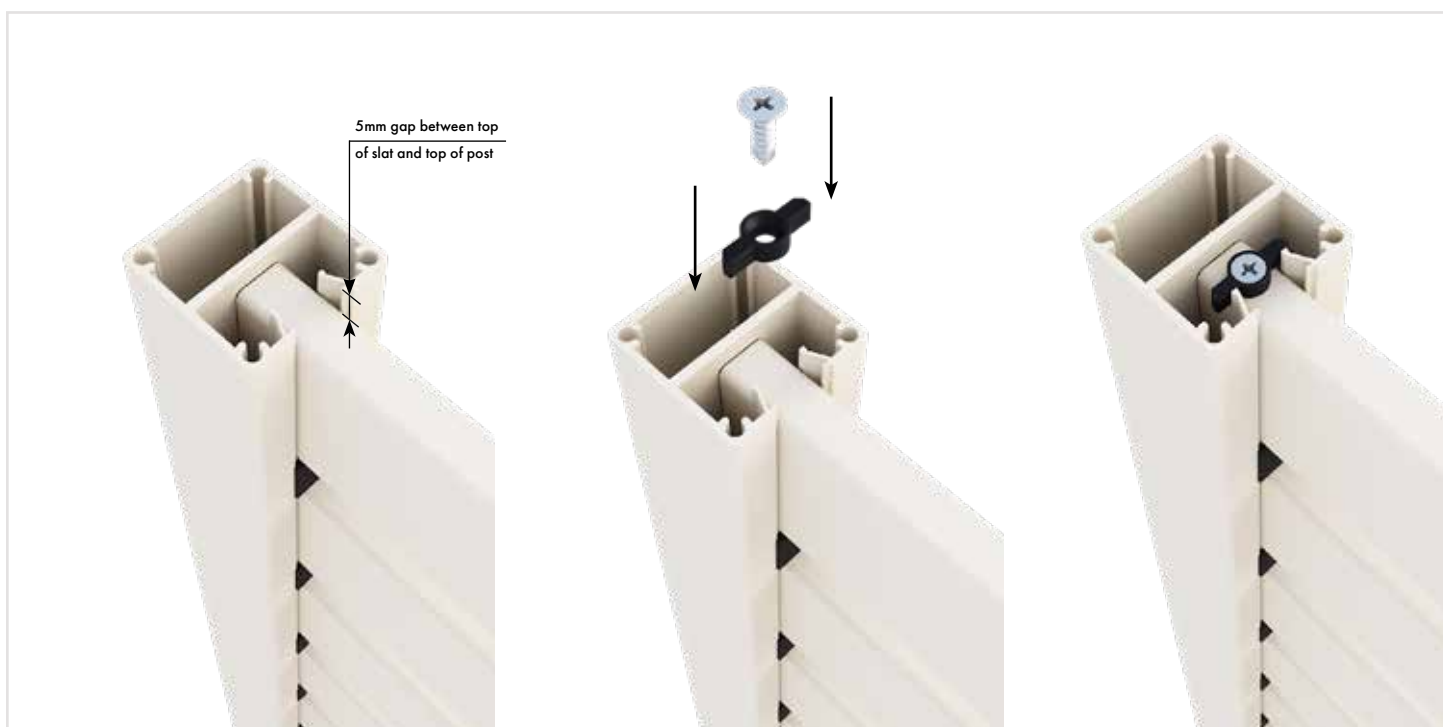
9 Top slat finishes 5mm below the top of the post. Screw slat locking clip into top slat.
