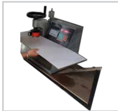
Carton cardboard tested for strength and breakage points. Thick cardboard is used for long term storage safety
