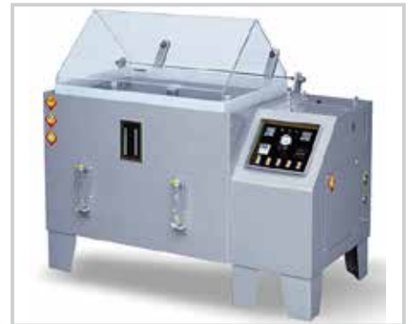
In-house salt spray testing - tests aluminium extrusion for durability of coating
