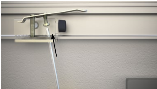
Adjust stopped tongue with second screw to desired clipping strength
