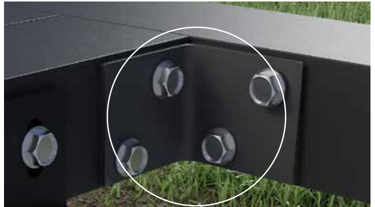
'Picture frame' ends if subframe not constrained between walls. Butt aluminium 55x40x3mm joist to ends of adjacent aluminium joists and secure in place with 40mm high angle
