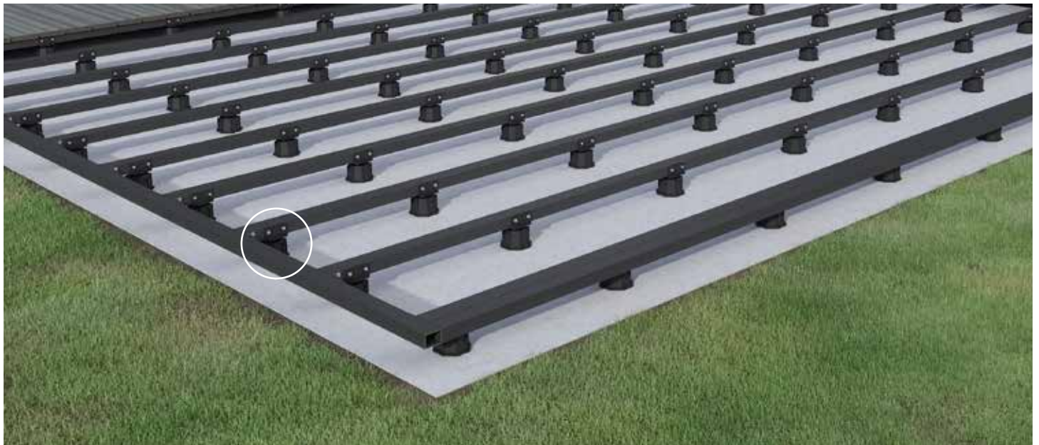
'Picture frame' ends if subframe not constrained between walls. Butt aluminium 55x40x3mm joist to ends of adjacent aluminium joists and secure in place with 40mm high angle
